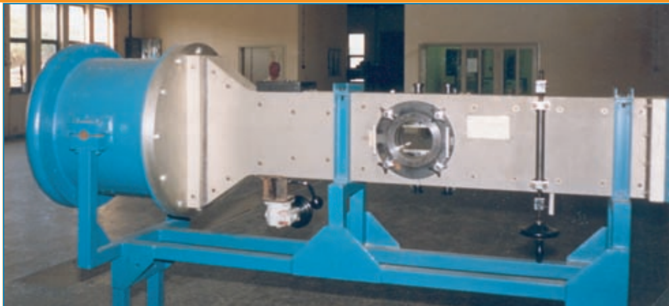
SMVS: 30 mm by 60 mm. Mach number continually variable during operation.
